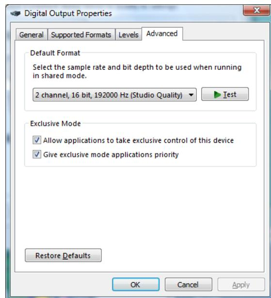
The selected sample rate (192 kHz) must match the sample rate setting made on the E-MU 0404 USB control panel.
