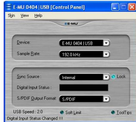
Unfortunately, the most recent firmware update of the E-MU 0404 / Tracker Pre does not save this setting, which means that you need to do this each time after powering on the unit.
