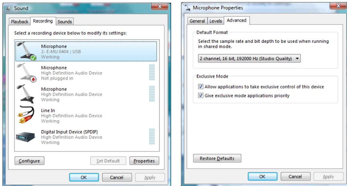
The selected sample rate (192 kHz) must match the sample rate setting made on the E-MU 04040 USB control panel.
