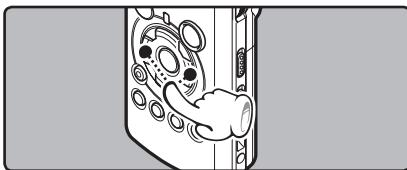
**While the recorder is during stop mode or playback mode, press the ▶▷I button.**
