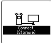
[Connect (Storage)] is appeared on recorder if the USB cable is connected
