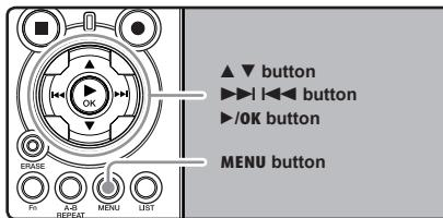
**1 While the recorder is during stop mode, press the MENU button.**
