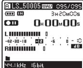
Example of conditions where the recording level has been lowered and the excess input has been adjusted
