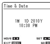
The clock will start from the set date and time. Press the ►/OK button according to the time signal.
