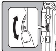
The volume can be adjusted within a range from [0] to [10]. The larger the number on the dial is the higher the volume will be.
