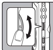
This can be adjusted in a range from [0] to [10]. The larger the number on the dial is the higher the recording level will be, and the indicator position of the level meter will grow larger as well
