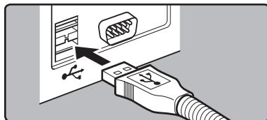
3 Confirm that the recorder has stopped and connect a USB connection cable to the connection port on the side of recorder.
