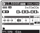
When the level meter is maxed out (the recorded sounds will be distorted)
