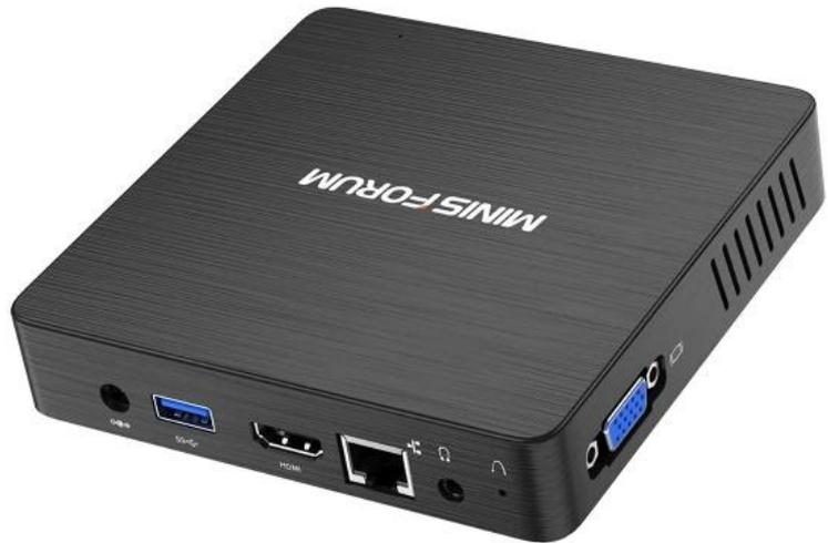
Fanless Intel Atom based mini PCs with 2 W scenario design power (SDP) specification are a good choice for this task. In combination with a single-channel UltraSoundGate 116xxx device running at a sample rate of 250 kHz they consume less than 3 Watt from a 12V lead acid battery.
