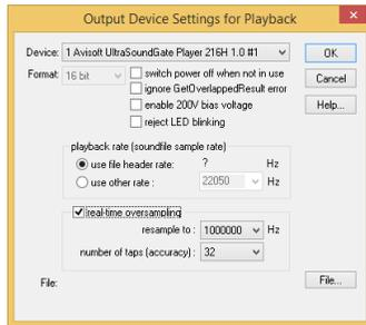
In the bus-powered operation mode, the option “**switch power off when not in use**” will reduce the current drawn from the USB while no file is being played (the power amplifier will be switched off between playbacks). However, switching on and off the amplifier at the begin and end of each file can create an undesired noise. If this noise is unacceptable, the option should be disabled.
