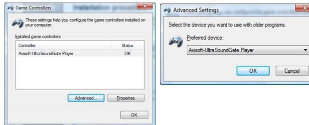
When simultaneously playing via the USG Player and recording via an UltraSoundGate xx16 at the same time, it is necessary to launch a separate instance of the RECORDER USGH software for the playback task. Otherwise, the recording and playback procedures might disturb each other (gaps might occur in the data streams).
