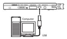
When connected to a computer, a pop-up window appears on this unit's display to let you choose whether you want to operate the unit using USB bus power or to connect the unit with the computer by USB.
