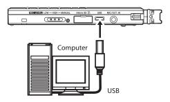
If you connect the unit by USB when its power is ON, or if you turn the unit's power ON when it is already connected by USB, a screen appears on this unit's display to let you choose whether you want to operate the unit using USB bus power or to connect the unit with the computer by USB.
