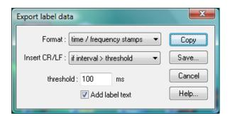
CR/LF control characters can be automatically inserted based on a time interval threshold in order to separate syllables. In case the individual syllables were too close to each other, the last measurement point of each syllable could be manually marked by entering a dot character:
