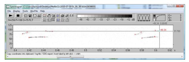
These manually placed labels represent the time and frequency of the marked point. The labels can be reviewed or edited (moved) afterwards and will be saved along with the .wav file. The coordinates of these labels can then be exported into an ASCII file or into the Windows clipboard from the main window command Tools/Labels/Export label data...:
