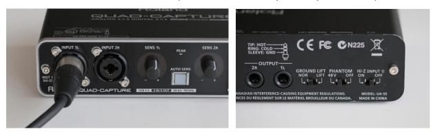
The USB audio interface has two microphone inputs (*INPUT 1L* and *INPUT 2R*). It is therefore necessary to attach the microphone to the correct input channel. This would usually be **INPUT 1L** if the (default) *left Channel* has been selected from the above Configuration dialog box of the RECORDER software.
