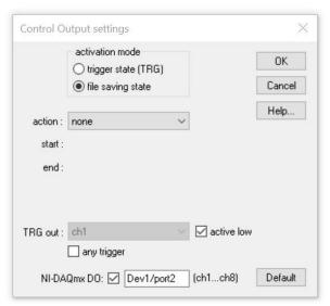
Then navigate to *Options > Control output settings...*, activate the *NI-DAQmx DO* option and select the NI device (*Dev1*) and port (*port0...3*) that should be used for sending the TTL pulse. The least significant line (PX.0) of the selected port will be linked to first channel in the RECORDER USGH NI-DAQmx software (PX.1 will be linked to the second channel and so on).
