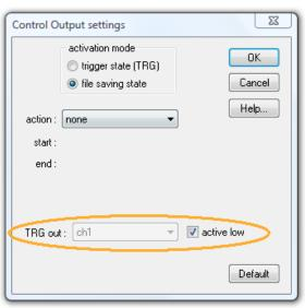
If the *file saving state* has been selected, the TRG output will be active as long as a .wav file is being saved onto disk (excluding the pre-trigger interval). Note that there will be a jitter of several 10 ms, depending on the selected *Buffer* size settings.
