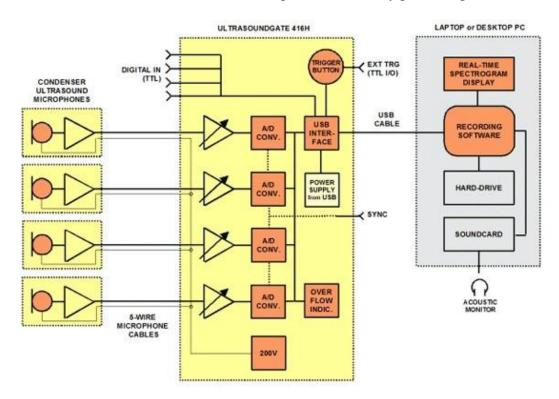
Advanced hardware and software options allow easy synchronization of USV and video recordings.
