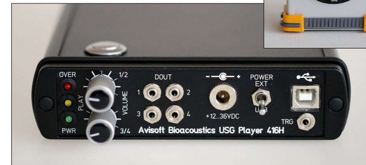
UltraSoundGate Player 416H (4 channel playback)
