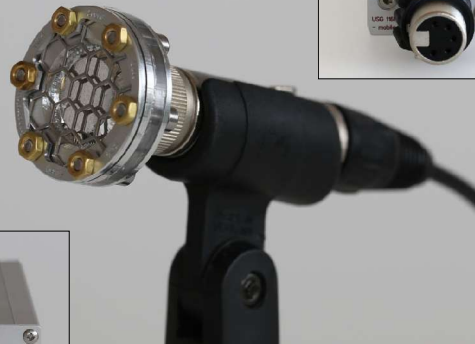
Very sensitive externally polarized solid-dielectric condenser microphone CM16/CMPA with a flat frequency response between 2 and 200 kHz.
