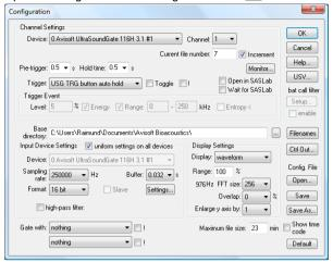
The input sample rate can be selected from the *Input Device Settings* section. Available sample rates are 750, 500, 375, 300, 250, 214, 187, 166, 150, 125, 100, 75, 62 and 50 kHz.
