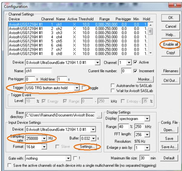
There is a list of 24 virtual channels at the top of the configuration panel. Each of these virtual channels can be assigned to a physical channel of the UltraSoundGate unit by selecting the desired **Device** and **Channel** number for each list entry. The button labeled "Enable all" will assign and activate all available channels automatically.
